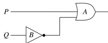
In problems 23–25, determine the final outputs for all possible inputs for each diagram.
