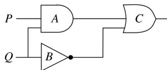
The output of  $A$  is symbolized by  $p \wedge q$ , and the output of  $B$  by  $\sim q$ . Thus, the inputs of  $C$  correspond to  $p \wedge q$  and  $\sim q$ . Since  $C$  is an OR gate, the final output can be symbolized by the statement  $(p \wedge q) \vee \sim q$ . If
